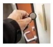
A security fob is a small device that wirelessly connects with your security system, activating or deactivating it. They work via Radio Frequency Identification (RFID), and are usually small enough to be kept on key rings, or in a pocket/wallet.
